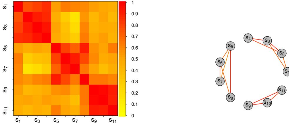
Figure 2: Left panel, heatmap of the correlation matrix of the sensor values ( $s_1-s_{11}$ ). Right panel, the undirected graph of partial correlation using the graphical lasso. The undirected graph of the right panel approves the block structure of the heatmap of the left panel.
